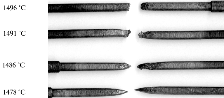
Fig. 5. Samples of cast carbon steel (0,22 %C) after testing at different temperatures
