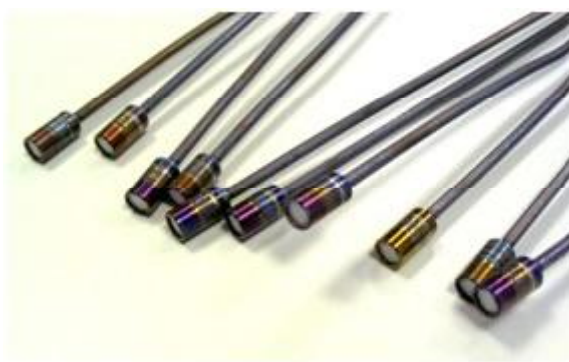
Figure 1. Picture of the ten microwave high temperature probes used for the engine test. Eight probes were mounted in the engine and two probes were used as spare
