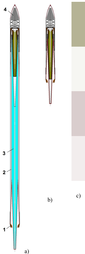
Fig. 2. The conceptual design of a portable pulse-inertial autophage launch vehicle: a) – initial configuration; b) – final configuration; c) – second stage separation; 1 – first stage conical shell spike engine; 2 – fuel; 3 – oxidizer, 4 – payload with attached second stage engine
